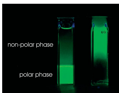
Figure 3. Oleylamine-driven phase transfer of nanocrystalline \text{LaPO}_4\text{:Ce,Tb} from the polar phase (A, e.g. methanol, ethanol, diethylene glycol) to a nonpolar dispersant (B, e.g. hexane, toluene).
